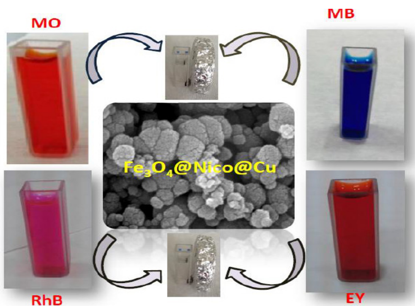
Figure 4.33: Photo that illustrates color change of azo dyes after catalysis reaction and easy separation of it by a magnet.
