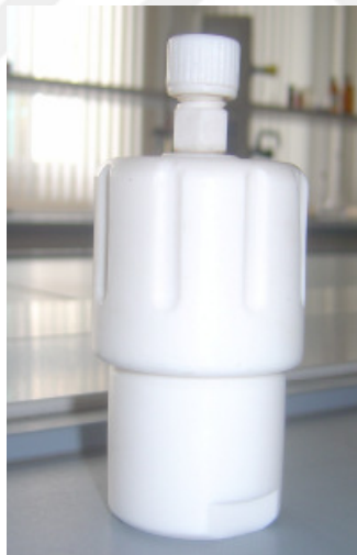
Figure 1.5: Autoclave used for hydrothermal method.
