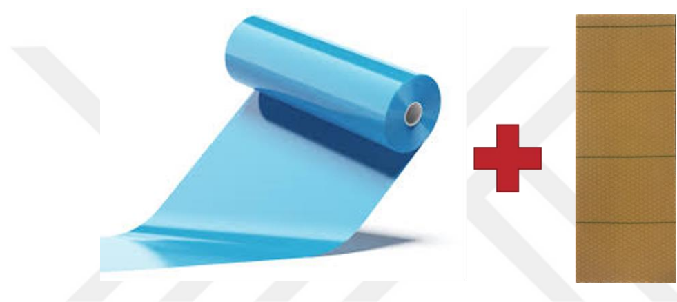
Figure 3.3 A representative illustration of embedding Teflon film into sample to create debonding
