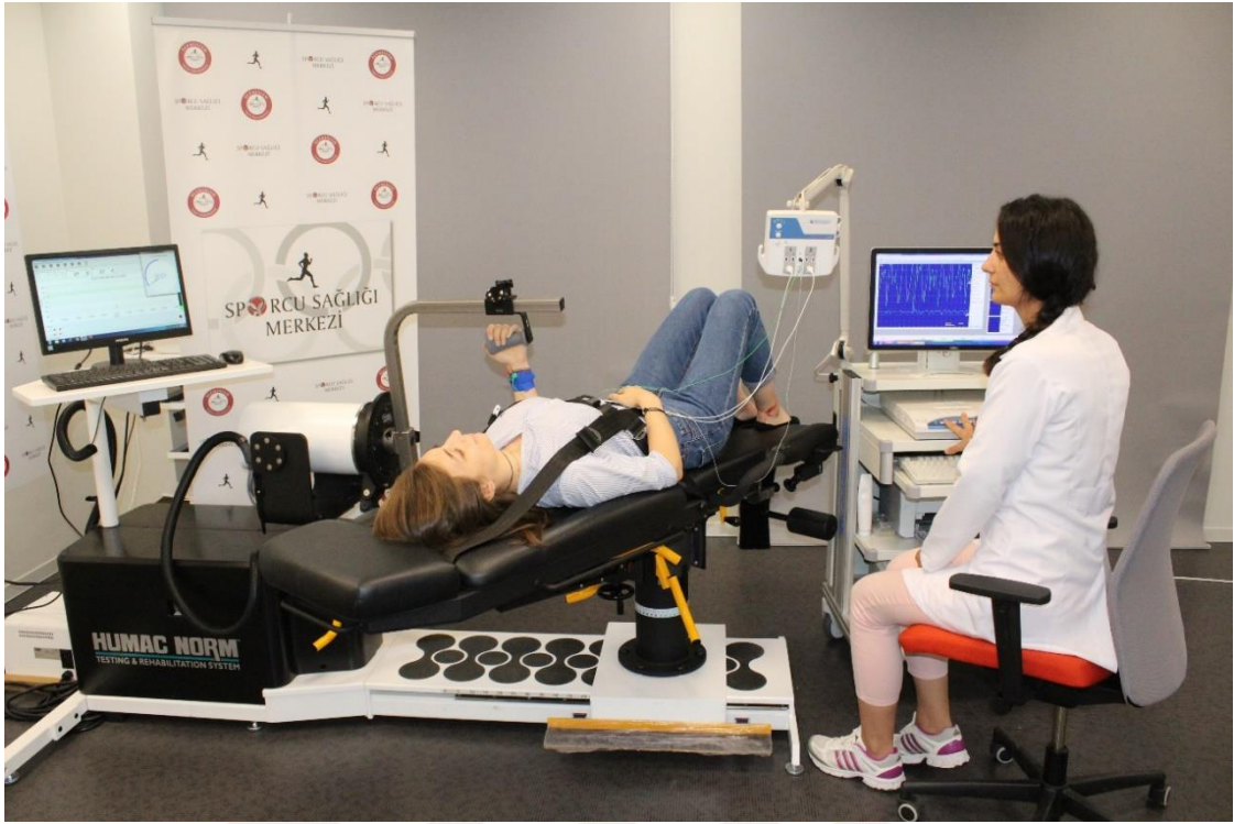
Figure 2.2: The gathering of maximum isometric voluntary contraction EMG of the left arm biceps and triceps brachii muscles.
