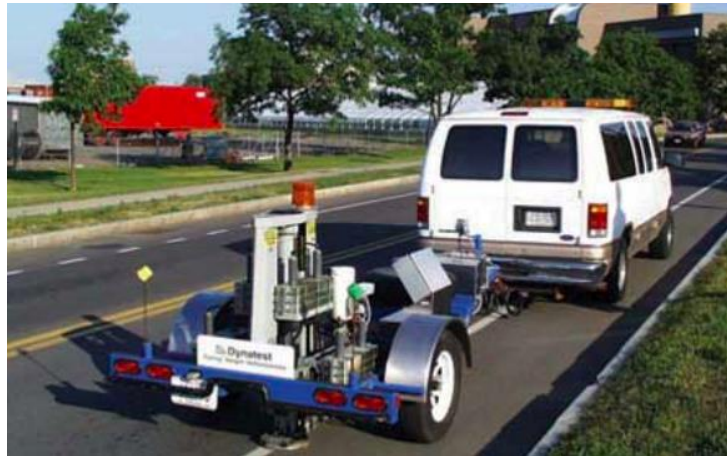
Şekil 2.16: FDW (Falling Weight Deflecometer) (URL-3)
