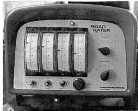
Figure 2 Road Rater Control Console
