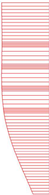
Fig. 6 Horizontal displacements in beam (plate no: 1)
