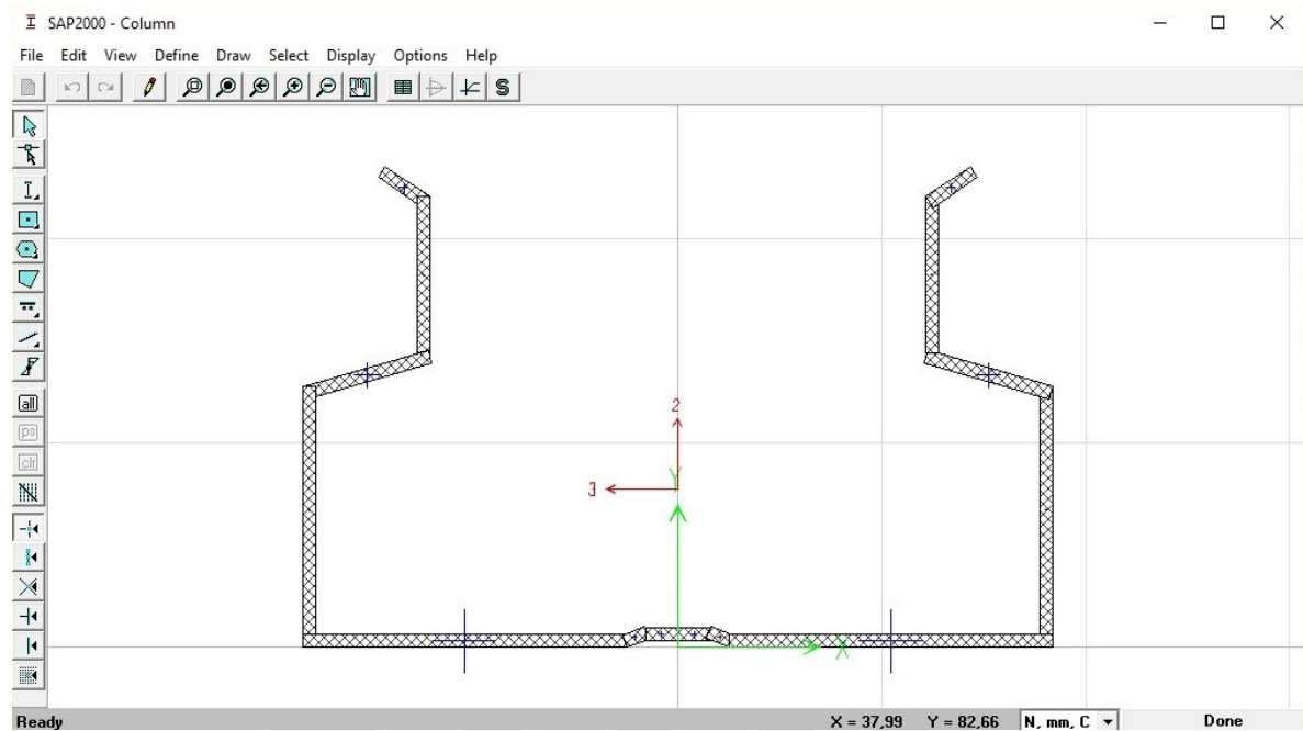
Figure 6.6: Defining the dimensions of the column using the section designer menu in SAP2000.
