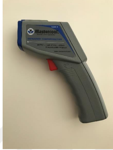
Resim 3.1. Temassız kızılötesi (infrared) termometre (Mastercool 52224-A Gray Infrared Thermometer with Laser®)
