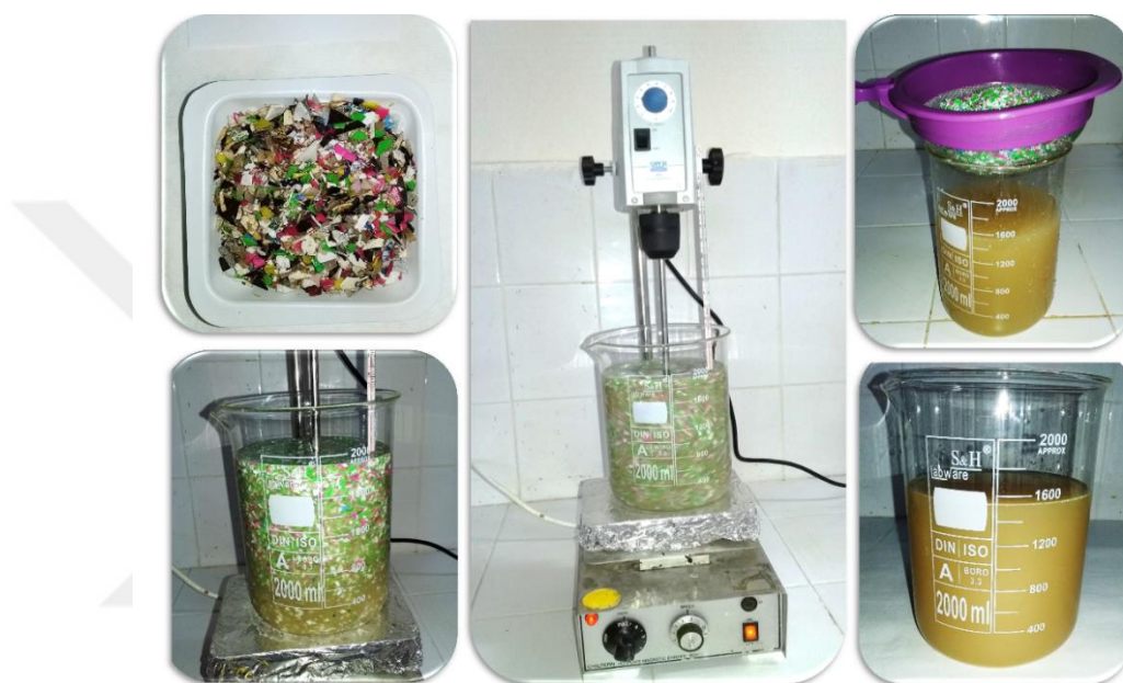
Figure 3.3. Waste plastic washing process
