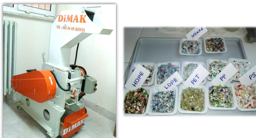
Figure 3.2. Laboratory scale plastic crushing machine and shredded plastics
