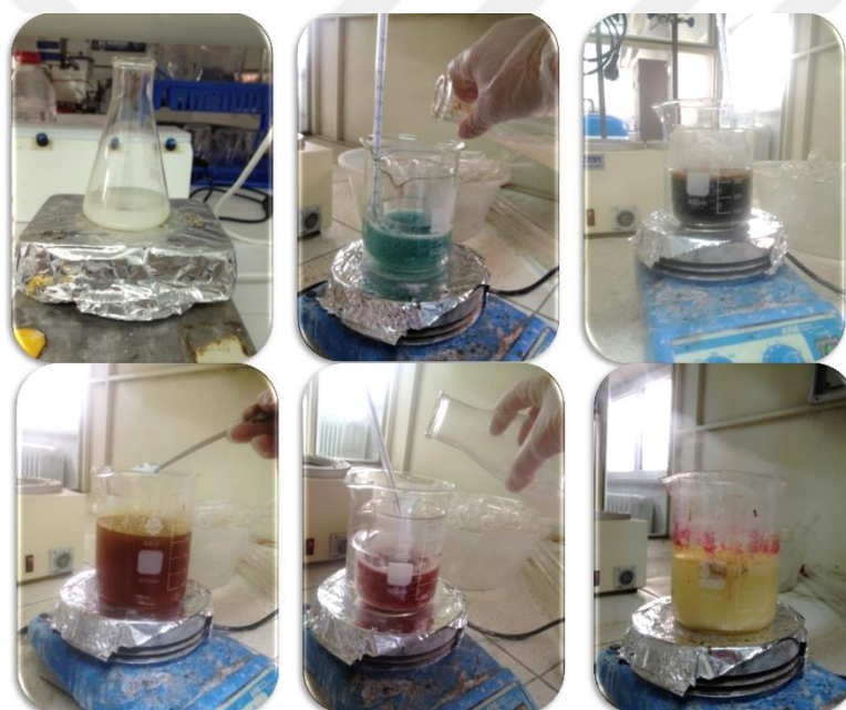
Figure 3.4. Steps of FSPS synthesis by classical method (Vink, 1981)
