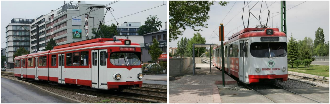
řekil 4.7. Duewag GT8, 3 b lmeli ve 5 kapılı tramvay modelin g r nt leri.(Wittenfeld 2006)
