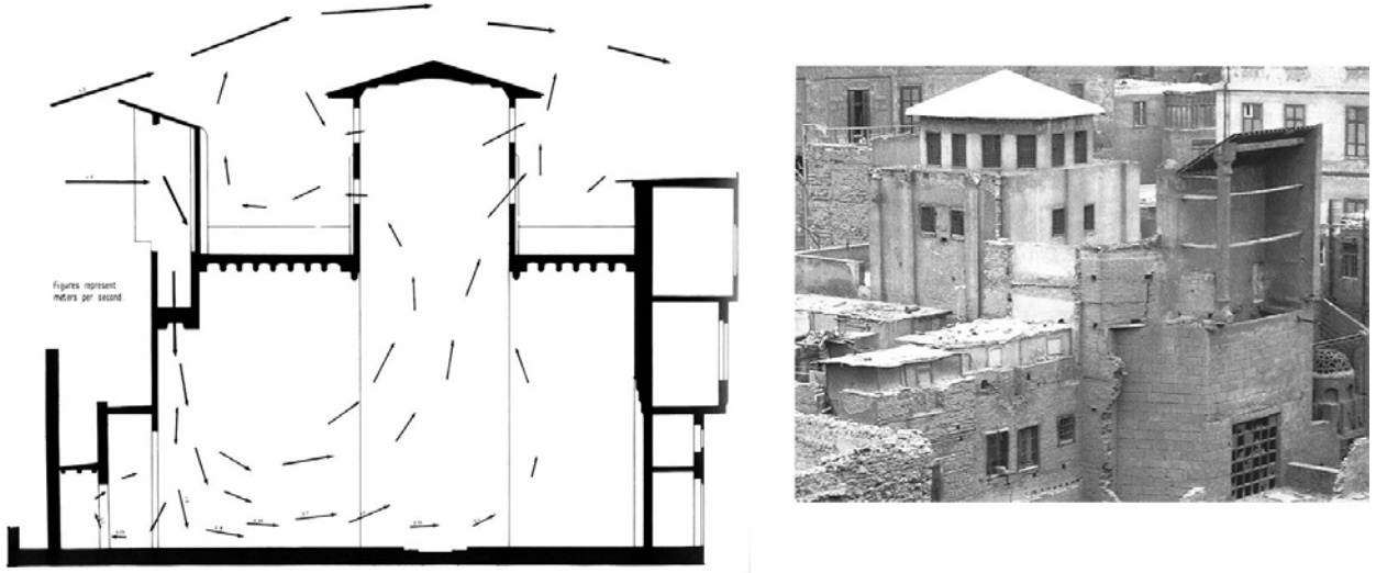
Şekil 5. Beyt Kethüda-Kahire, 15.yy, , 'Malkaf' ve 'Shukshaykha' işleyiş diyagramı, STEELE, James; (1997), An Architecture For People: The Complete Works Of Hassan Fathy , Whitney Library Of Design; An Imprint of Watson-Guption Publications, New York, s.176-177
