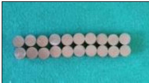
Figure 18: The Sandblasted Ti alloy disks
