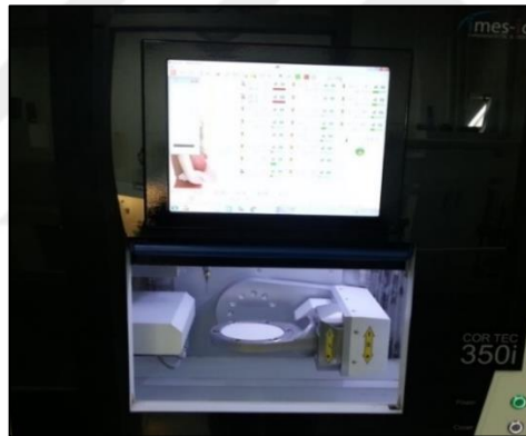
Figure 4: Milling of titanium disks in cad/cam machine
