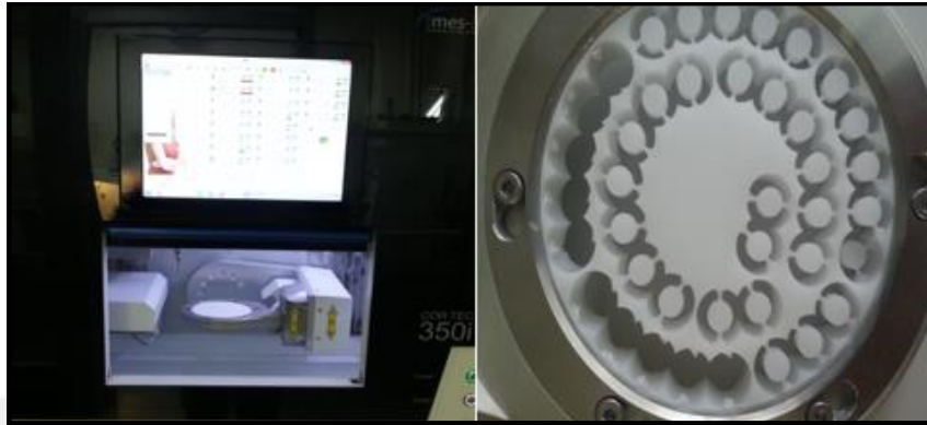
Figure 8: Cutting of wax by cad/cam system
