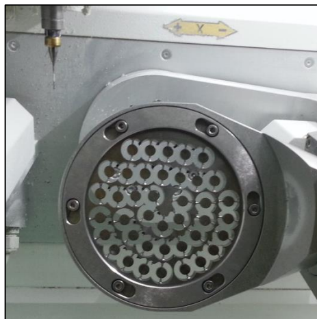
Figure 5: Titanium disks after cutting
