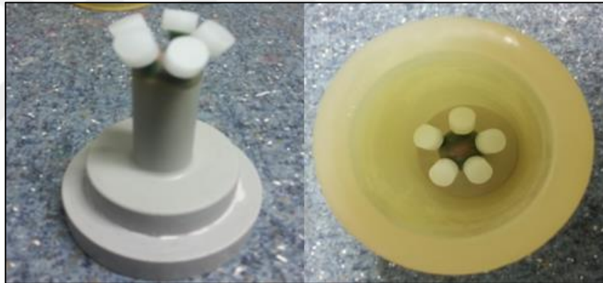
Figure 9: Spruing of wax disks
