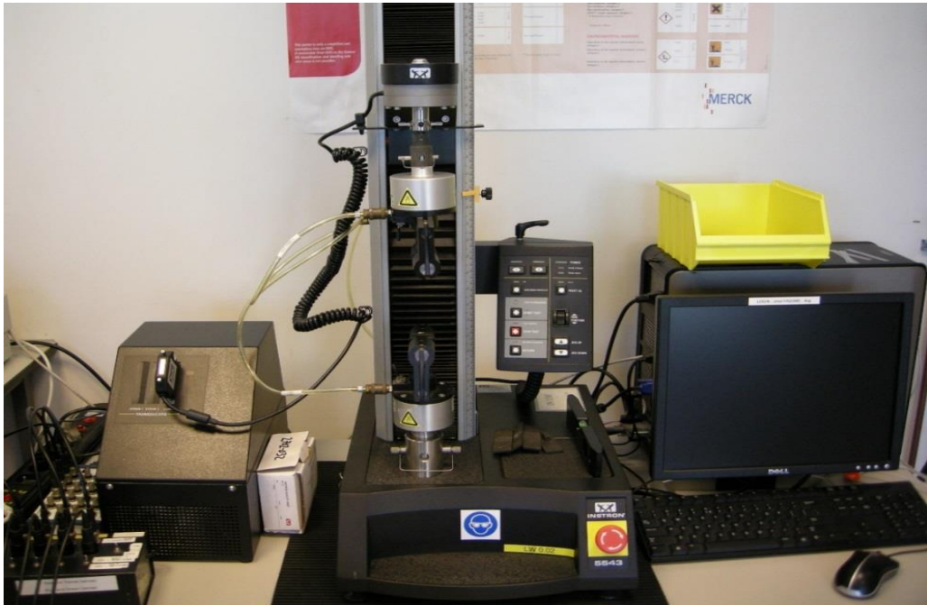
Figure 2.14: Laboratory set-up: Instron Universal Testing Machine.
