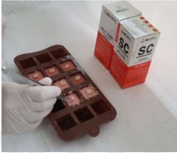
Figure 4: Embedding of specimen in self-curing acrylic resin.
