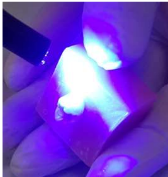
Figure 18 : Curing for 10 seconds.
