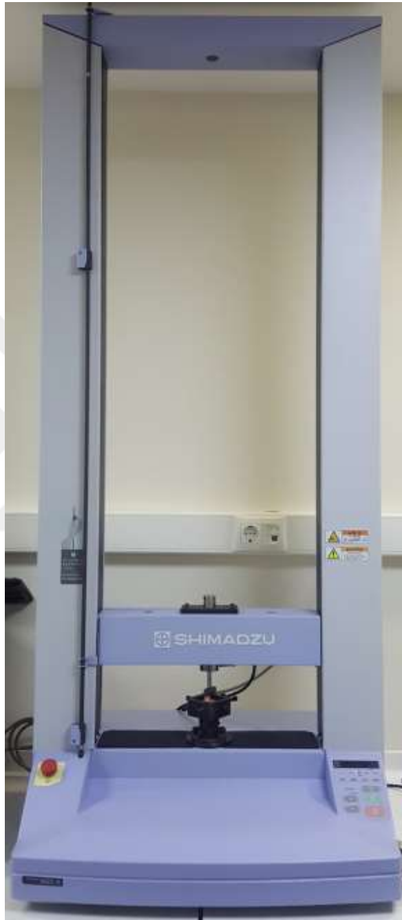
figure 20: Testing the shear bond strength by universal testing machine.
