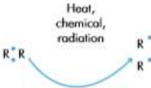
Figure 2: Illustration of external energy factors acting on a radical-generating component to form free radicals
