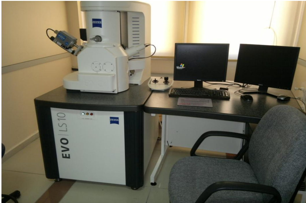
Figure 3.4. This SEM and EDX used for analysis.
