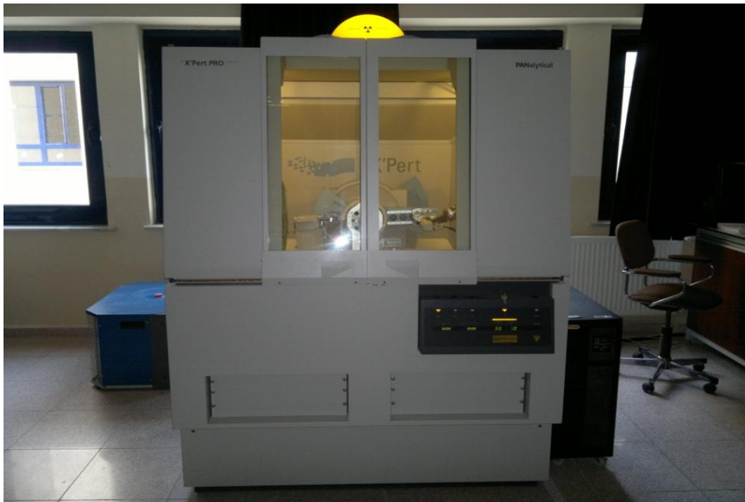
Figure 3.3. This XRD used for analysis.
