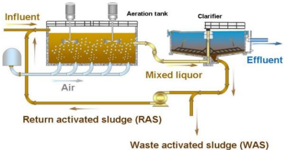
Figure 2.2: The operation of activated sludge processes
