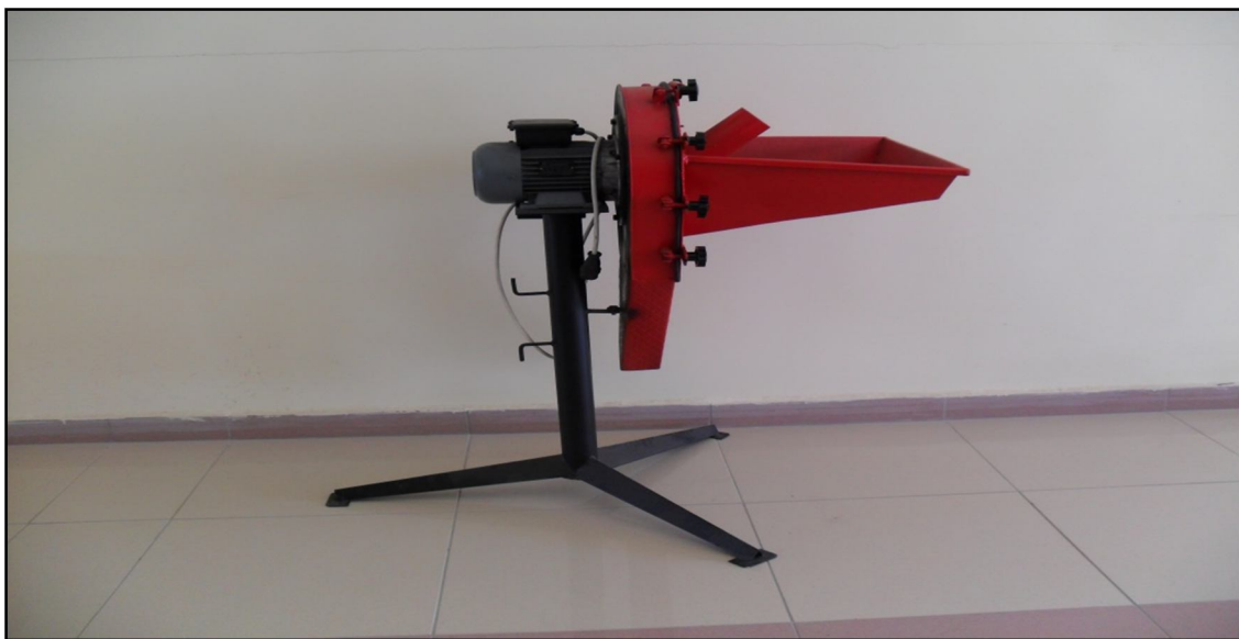
Figure3.8.The mill used for grinding oak acorn and other feed ingredients
