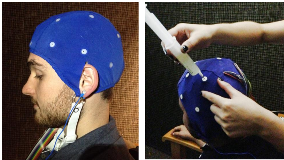
Fig. 4.1 :EEG preperation. Left figure shows the placement of the 10-20 system EEG Headcap. Right figure demonstrates the filling the electrode-tissue interface with conductive gel.
