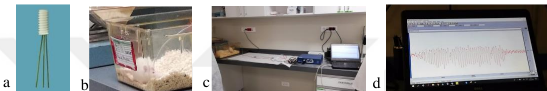
Figure 22. (a) Cortical EEG recording was achieved with three channel electrodes; (b) the electrodes were connected to EEG system; (c) Biopac MP36 system was recruited; (d) Half an hour baseline activity revealed the characteristic SWD oscillations in WAG-Rij.
