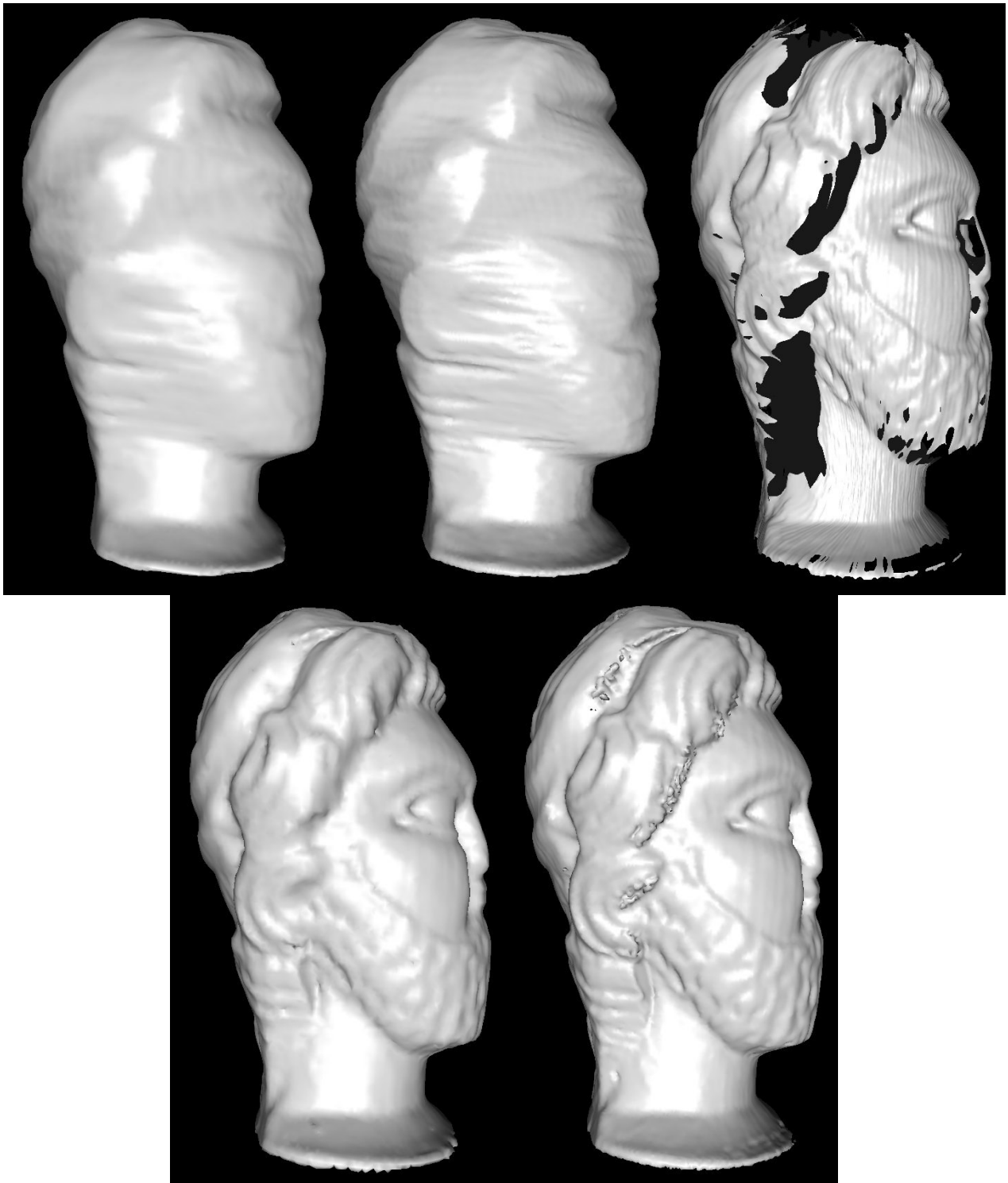
Figure 6.9: More views of the reconstruction of the Greek1 model. Starting from the top left: Silhouette reconstruction ( R = 7 ), Silhouette reconstruction ( R = 8 ), Optical triangulation, Fusion ( R = 7 ), and Fusion ( R = 8 ) are depicted.
