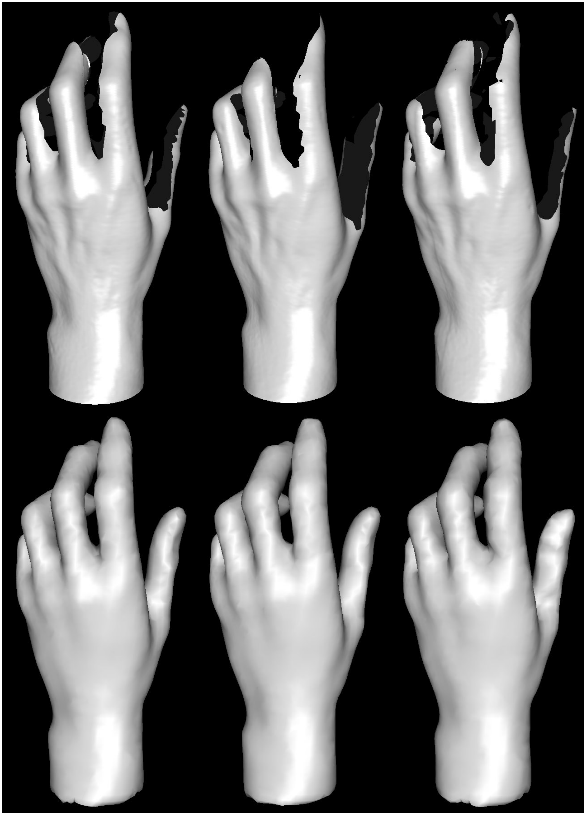
Figure 6.12: More views of the reconstruction of the Hand model. (Top row) First, second and third optical triangulations. (Bottom row) fusion of the silhouette reconstruction ( R = 7 ) with the first, second and third optical triangulations respectively.
