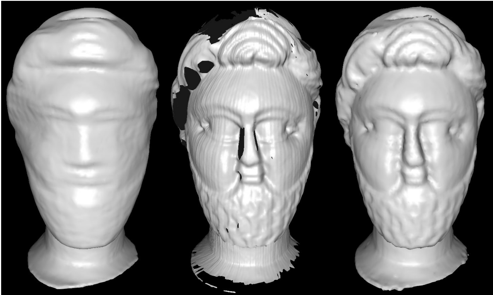
Figure 6.2: Reconstructions of Greek1 model. Each rendering is Gouraud-shaded. (Left) Silhouette model of resolution R = 7 after decimation. (Middle) Structured Light model after fairing. The traceable marks of the laser stripes on the object surface are a result of miscalibration and noise. (Right) Fused model at R = 7 resolution after decimation. Note the slight blurriness in the fusion due to insufficient depth of traversal in the octree.
