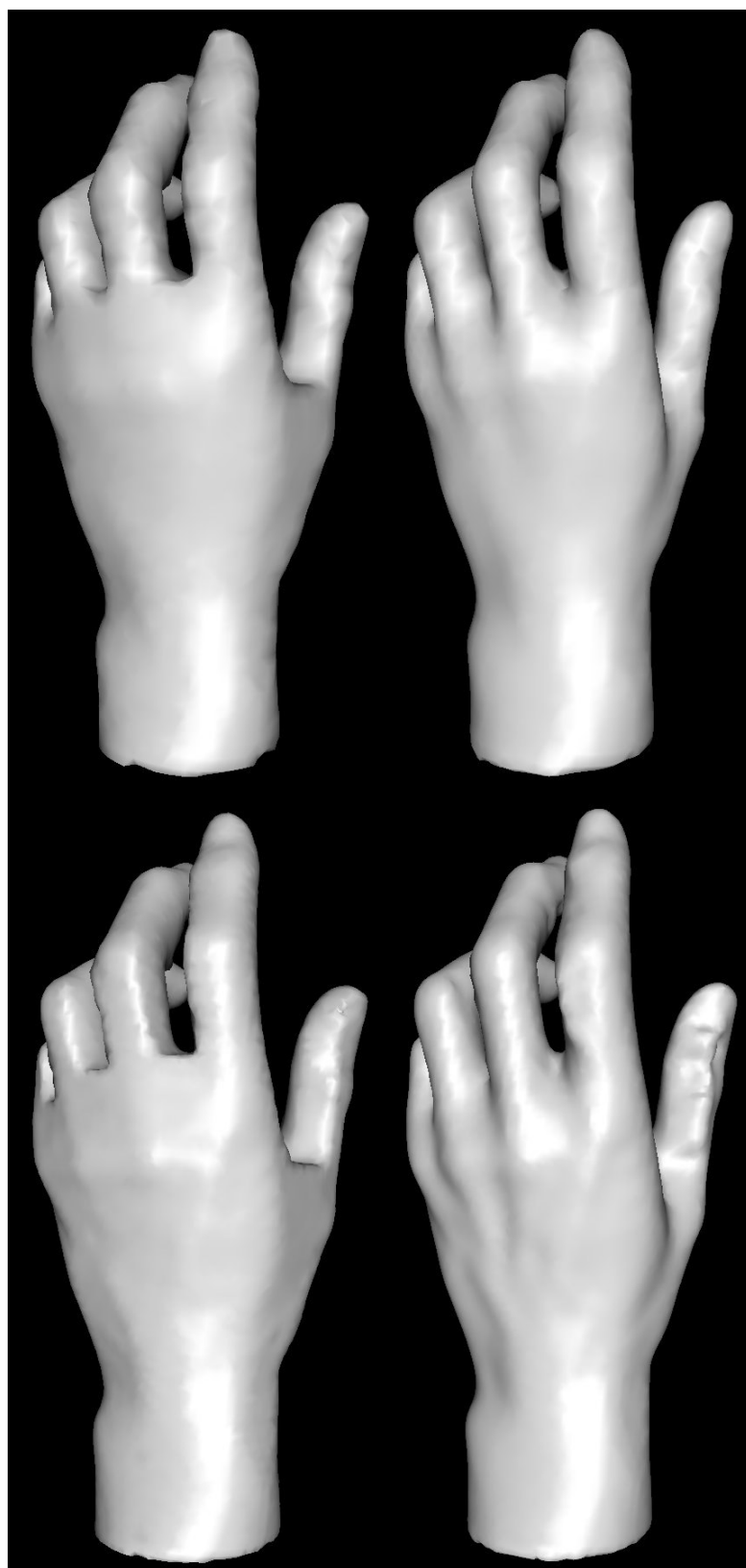
Figure 6.13: More views of the reconstruction of the Hand model (continued). Starting from the top left: silhouette reconstruction at resolution R = 7 , fusion at resolution R = 7 using the combination of three optical triangulations, silhouette reconstruction at resolution R = 8 , and finally the fusion at resolution R = 8 using the combination of three optical triangulations.
