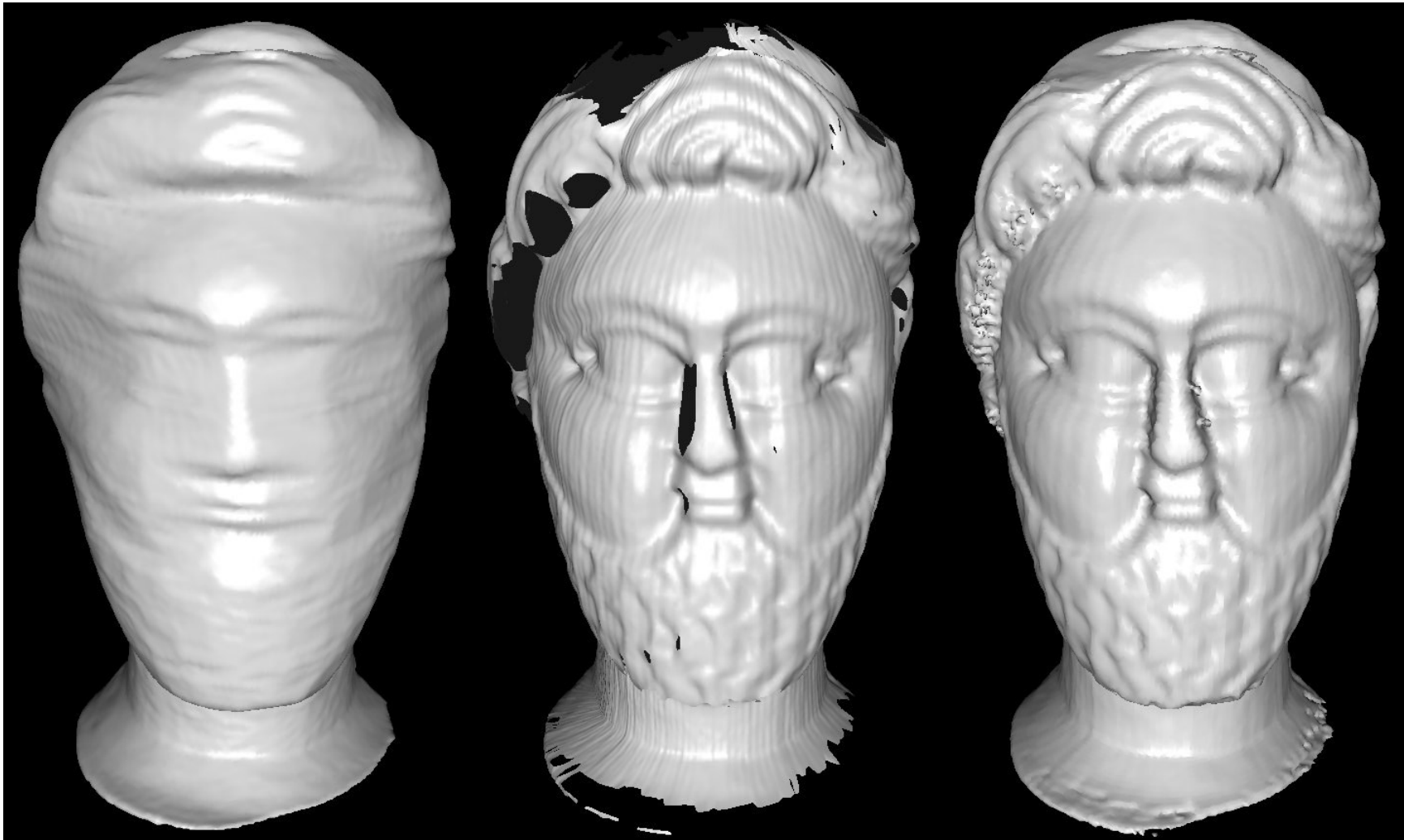
Figure 6.3: Reconstructions of Greek1 model continued. Each rendering is Gouraud-shaded. (Left) Silhouette model at resolution 8 after decimation. (Middle) Structured Light model after fairing. (Right) Fused model at resolution R = 8 . Note the overhanging irregularities beside the nose and below the hair line where the scan lines are too sparse to carve away the volume. The bumpy surface on the base of the fused reconstruction originates from miscalibration which mostly tends to cause misalignment of the scannings to materialize on the top and bottom sections of the fused reconstruction.
