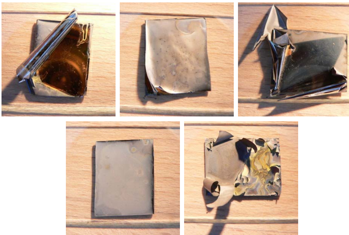
Figure 4-20 Some of the early attempts of electroplating. Most of them suffered from high residual stresses and peeled from the sides.
