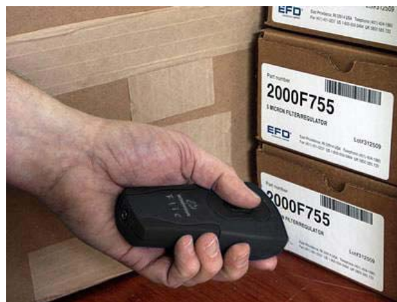
Figure 1-3 A hand-held laser scanning barcode reader (Photo courtesy of Microvision, Inc)
