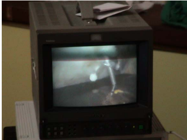
Figure 5.2: Video screen showing the pig liver and the indentation probe. The orientation and the position of the indenter were adjusted so that the probe was always perpendicular to the surface of the liver
