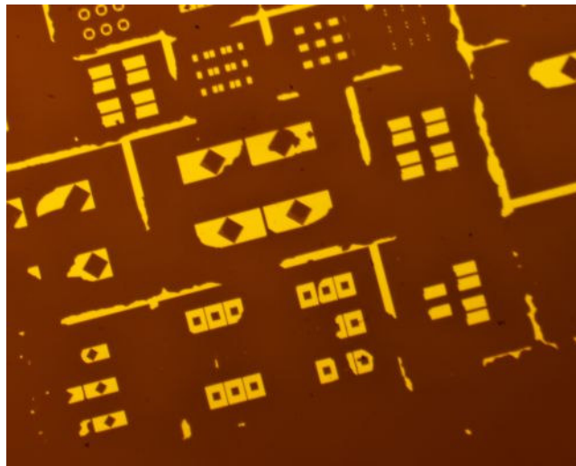
Fig.6.1 General View of Pyrex wafer after lift-off process
