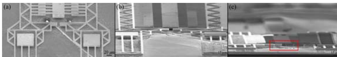
Figure 5.40 SEM images showing (a) 45^\circ (b) 80^\circ and (c) 89^\circ tilted front views of a pair of nanotweezers with nano-scale end-effectors in the form of merged nanoribbons after complete release
