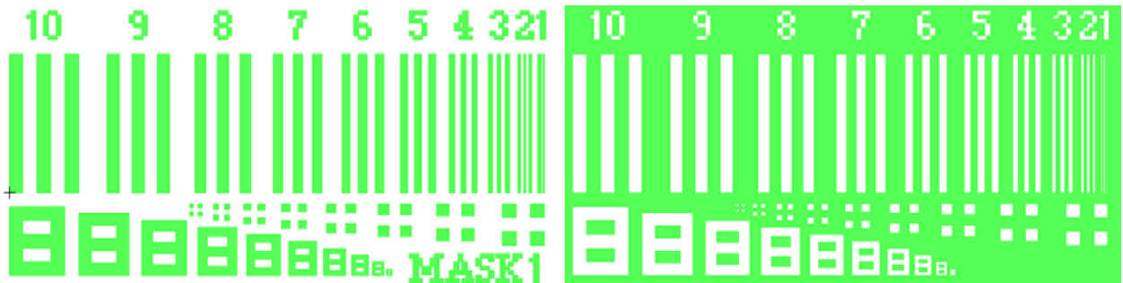
Figure 3.9 Lithography test patterns on Mask #1
