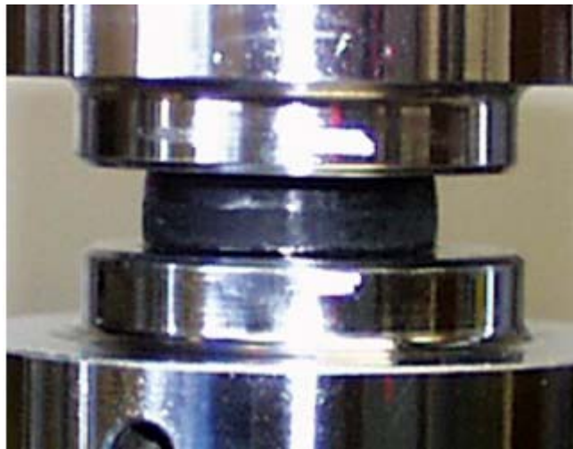
Figure 4.4: A lubricated compression specimen showing lateral constraining from friction [19]
