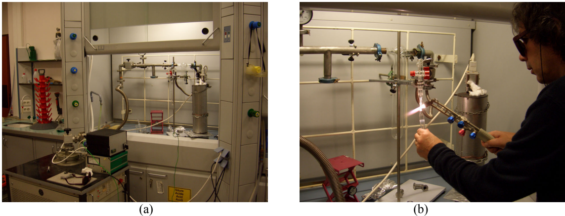
Figure 2.2: (a) Photograph of the vacuum line, (b) Prof. Mehmet Somer while closing the silica ampoule under high vacuum.
