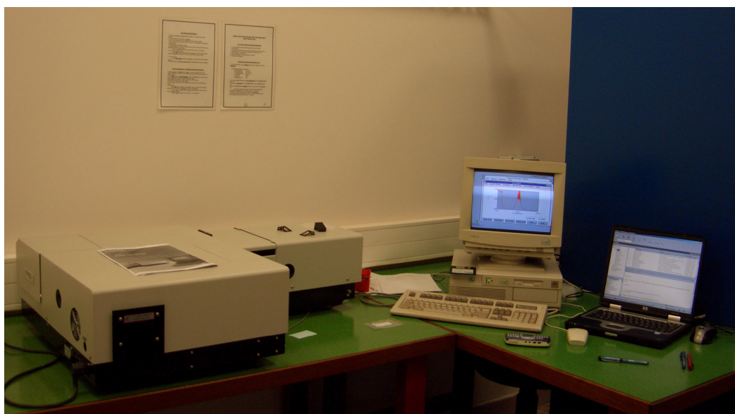
Figure 2.13: Shimadzu spectrophotometer that was used in the optical transmission and absorption measurements.
