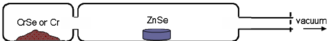
Figure 2.1 Schematic of the silica ampoule used in the preparation of \text{Cr}^{2+}:\text{ZnSe} by thermal diffusion doping.
