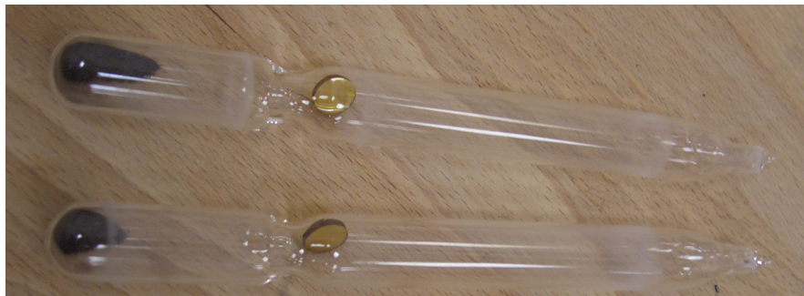
Figure 2.3: Sealed silica ampoules, containing pure ZnSe tablets and powder CrSe dopant, ready for thermal diffusion doping.
