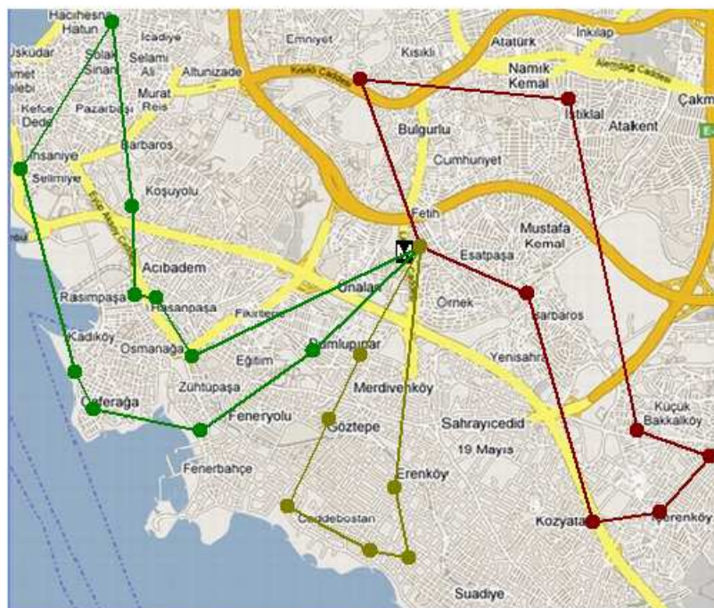
Figure 3.5: Optimization of grouping and delivery routes for 3 vehicles starting from a particular store. The greedy algorithm in which the nearest points are always preferred (upper). Optimized route (bottom) gives %40 efficiency compared to greedy algorithm , and distances are calculated as given in Eq. (3.1).
