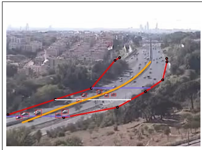
Figure 2.3: Road equation, shown as the orange curve, is extracted from the mask of detection region.
