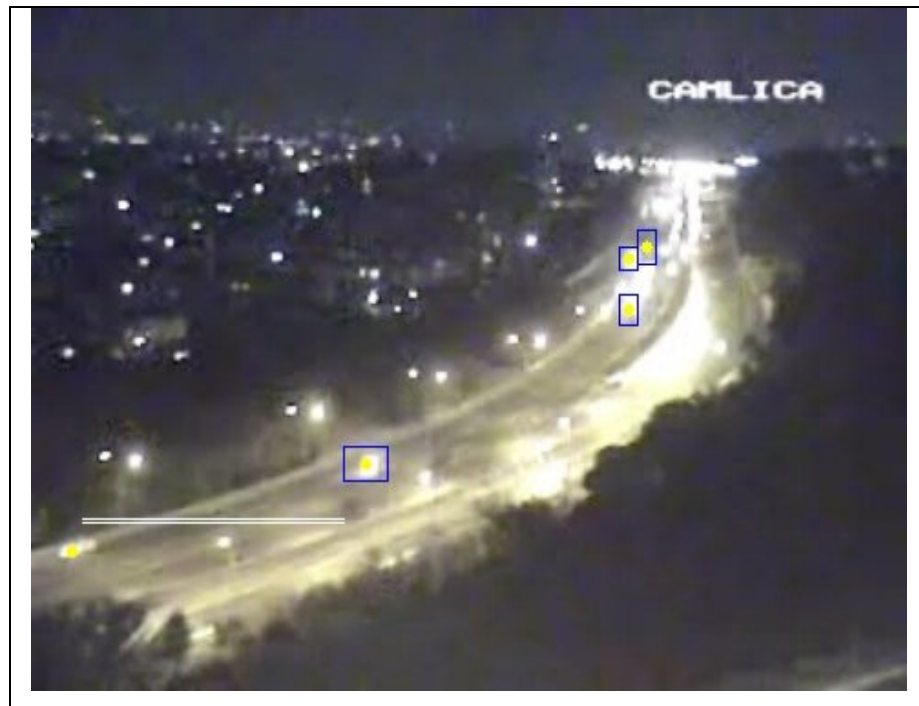
Figure 2.4: The white solid line represents the lower limit of the tracking boundary whereas yellow dots represent tracked vehicles and blue rectangles are detected vehicles.
