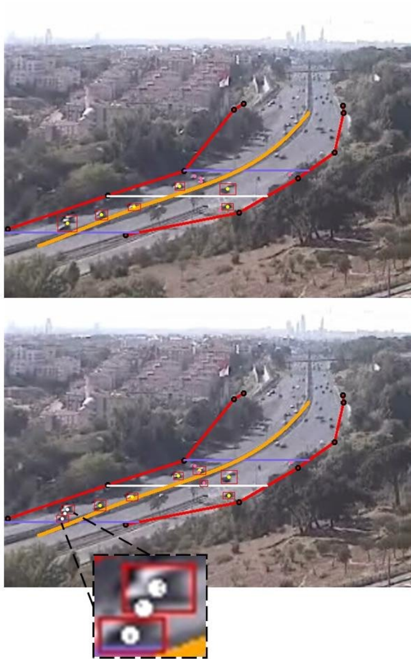
Figure 2.9: Split decision. Vehicles that are split and their previous position are detected as white dots.
