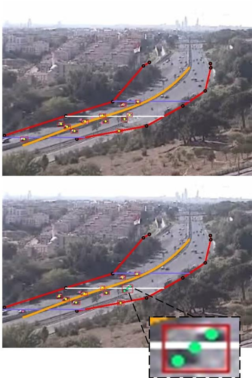
Figure 2.8: Occlusion decision. Occluded vehicles end rectangle center is represented with green dots.
