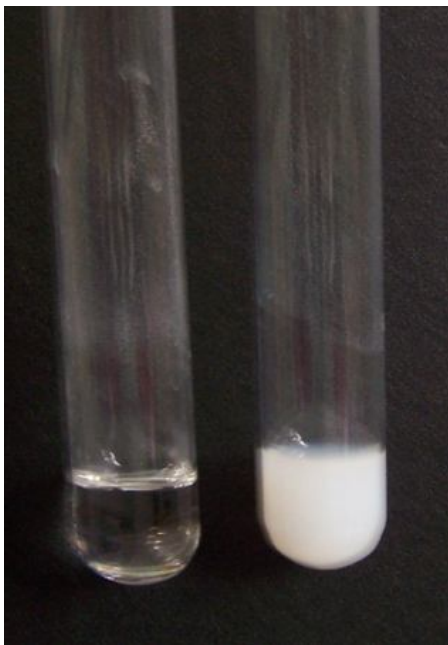
Figure 4.1: Dispersion of tin(IV)oxide nanoparticles in MMA after sonication for 15 min: without surfactant (left), with surfactant (right)
