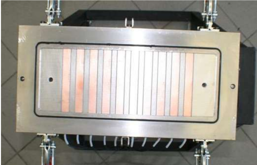
Lower mold plated with 6mm spacer frame.
