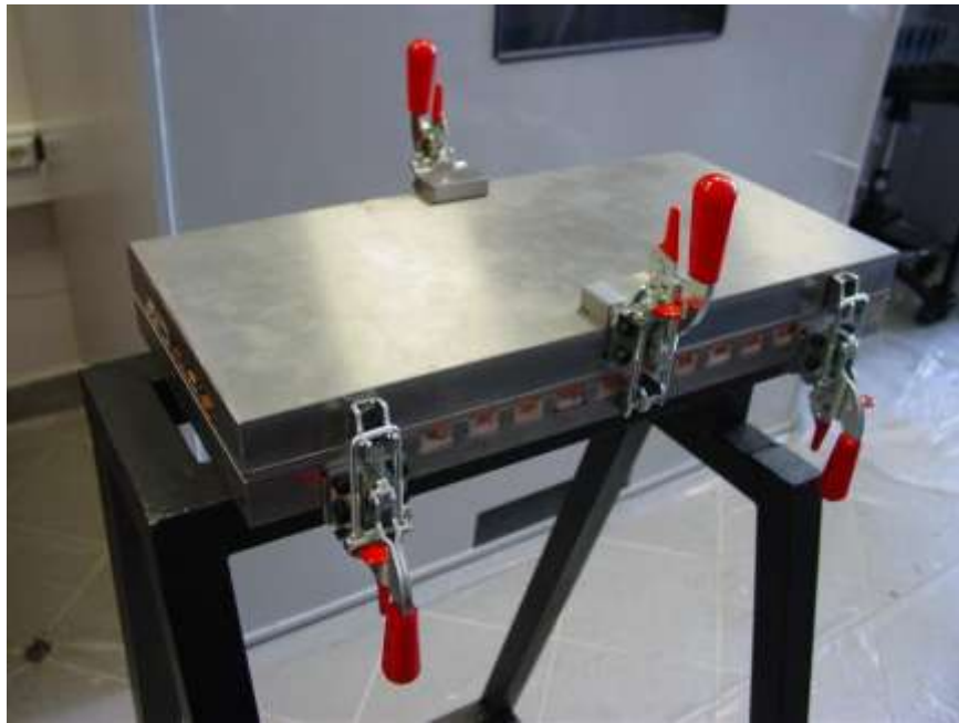
Mold with latches closed. Isometric view.
