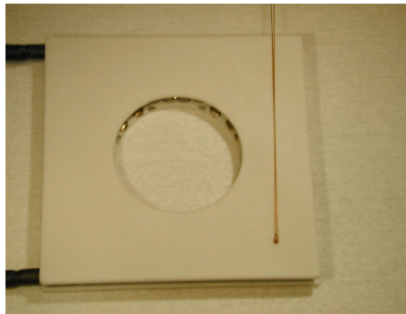
Figure 3-11 TEC (Melcor SH1.0-95-05L and thermistor (Shibaura Electronics PB7-43-SP2).
