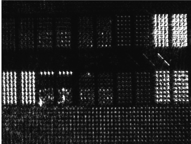
Figure 5-7 A snapshot of imaged first diffraction orders taken by CCD camera. The test die is composed of different designs with groups of 8 \times 4 and also includes an array of 10 \times 80 pixels. The first order diffracted light from each group shows different intensities.
