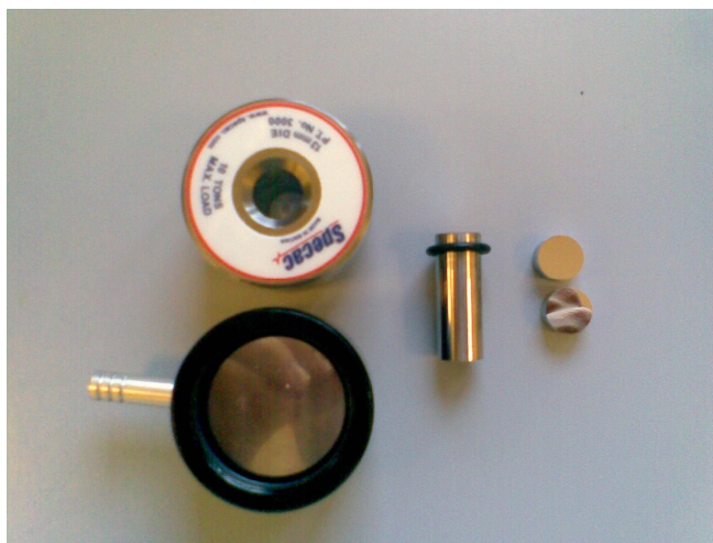
Figure 2.3 Setup for preparing 13mm pellet for IR measurement
