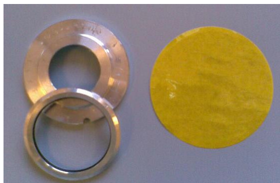
Figure 2.2 X-ray sample holder and Polyimide (Kapton ® ) film for moisture sensitive samples
