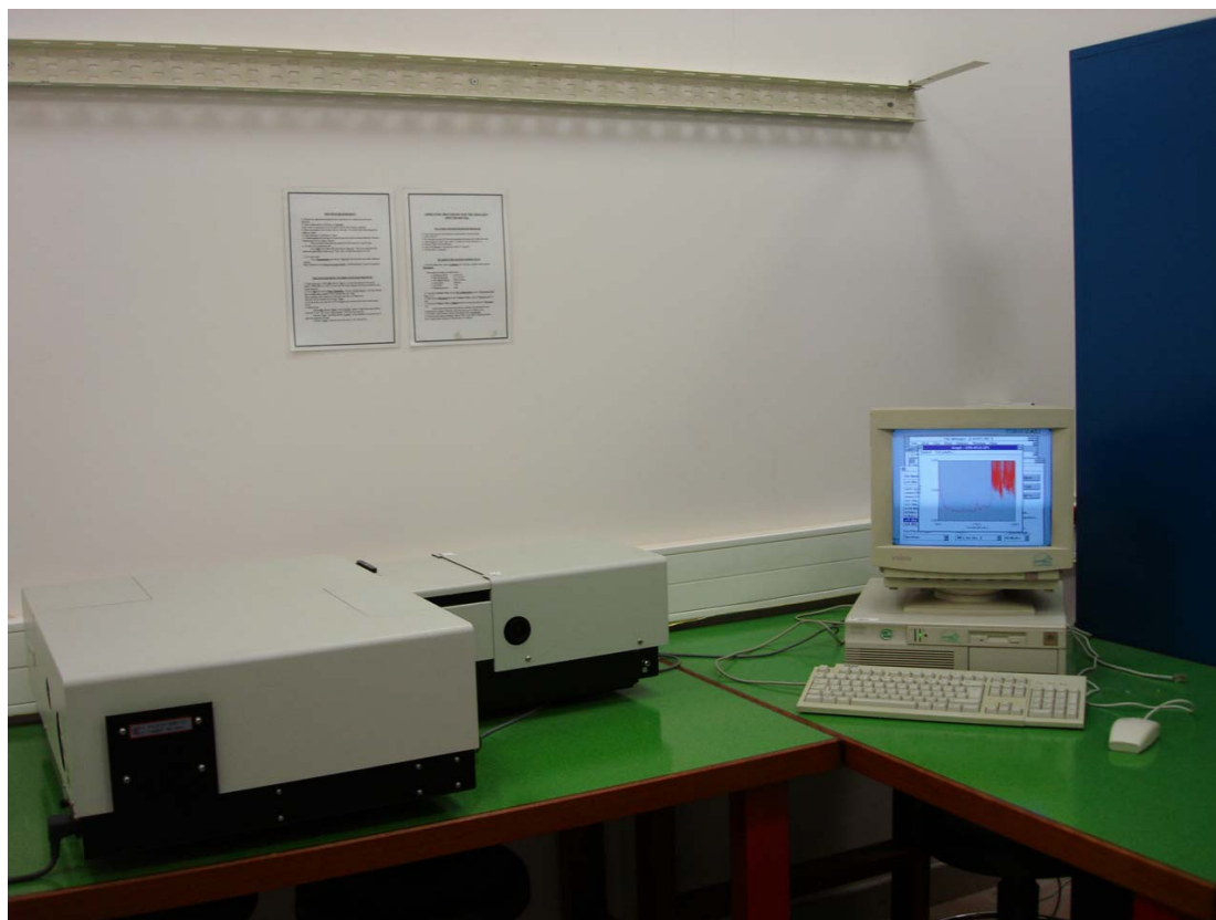
Figure 3.2: Shimadzu spectrophotometer for taking absorbance measurements.
