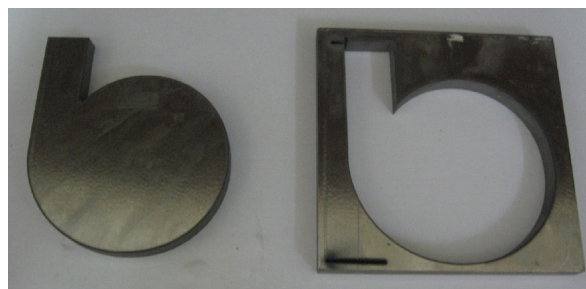
Figure 5.7: The outer profile of lower casing processed by a water-jet
