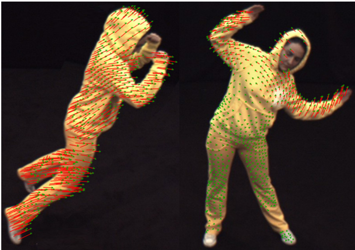
Figure 4.12: Sample frames with computed 2D optical flows. (Left) View from the 8 th camera at frame t = 748 and (right) from the 2 nd camera at frame t = 1040 .
