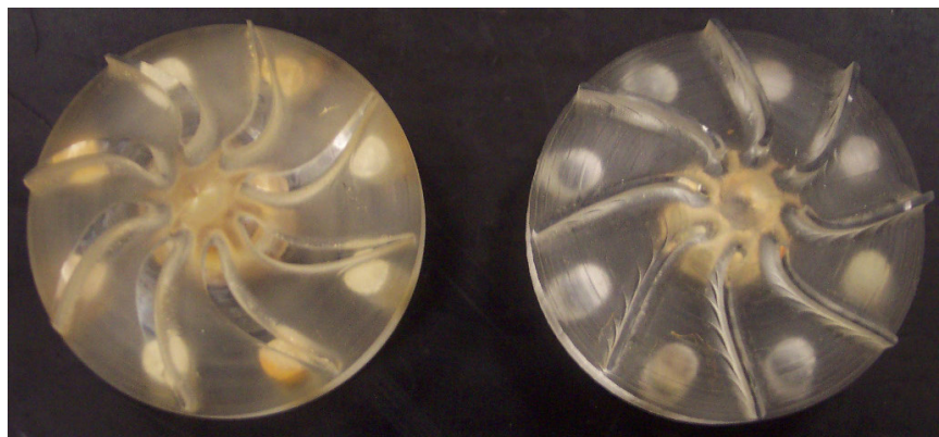
Figure 5.27: Airfoil Shaped and Constant Thickness Blade Impellers
