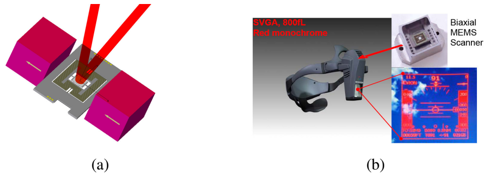
Figure 1.4: (a) Torsional microscanner with coils and magnets for a moving-coil actuator. (b) Nomad TM personal display system [6].
