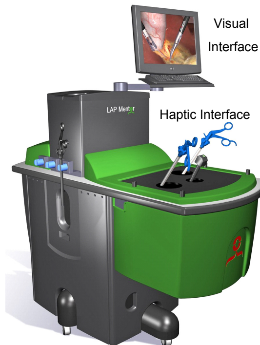
Figure 2. 1: Components of a typical minimally invasive surgery simulator (the Simbionix LAP Mentor laparoscopic surgery simulator) include a visual display and surgical instruments fitted with haptic devices for force feedback [1]
