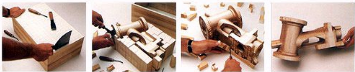
Figure 2. 40: The waste material is detached from the part by the help of the hatched areas [ http://home.att.net/~castleisland/faq/faq220.htm ]
