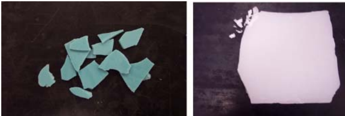
Figure 3. 28: Injection wax (left) and paraffin (right) were also tested in Design B besides the silicone
