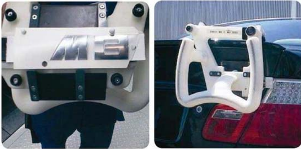
Figure 2. 61: This tool is used to affix the rear name badge
