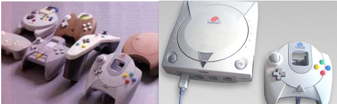
Figure 2. 46: a) Shape models of Sega game console's controller; b) one of them was chosen and produced
