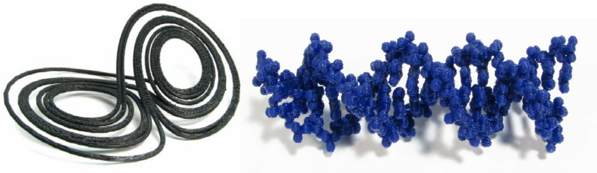
Figure 2. 53: A Lorenz attractor model (left) and a DNA strand model (right) which were produced by using an RP machine
