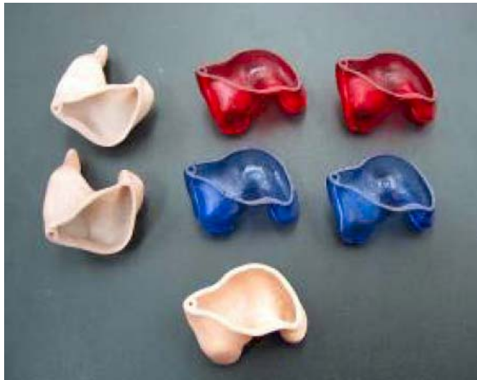
Figure 2. 62: Hearing aid shells produced by using SL machine of the 3D systems [ http://www.3dsystems.com/newsevents/newsreleases/pdfs/102004_3D_Systems_Introduces_New_Hearing_Aid_Shells_MFG_System.pdf ]
