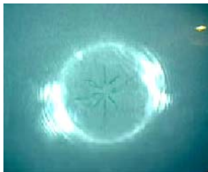
Figure 1.2 Raman lasing from pure water
