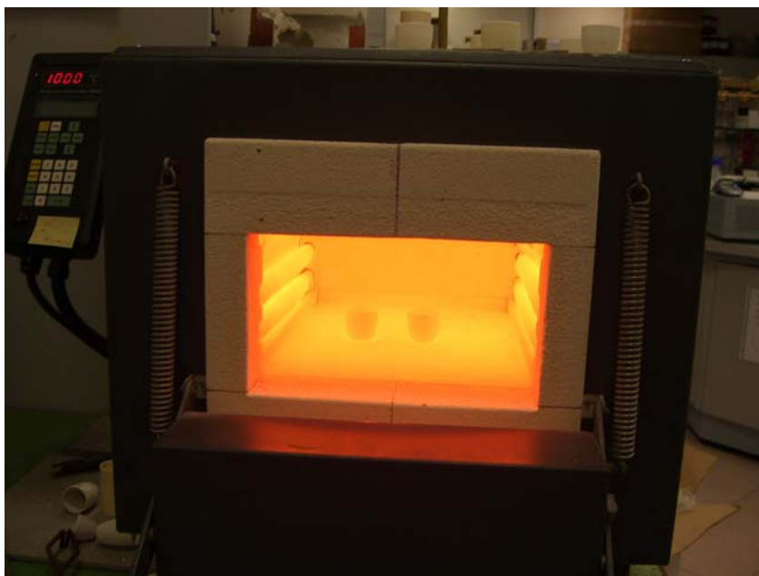
Figure 2.4 Annealing process in the muffle furnace.
