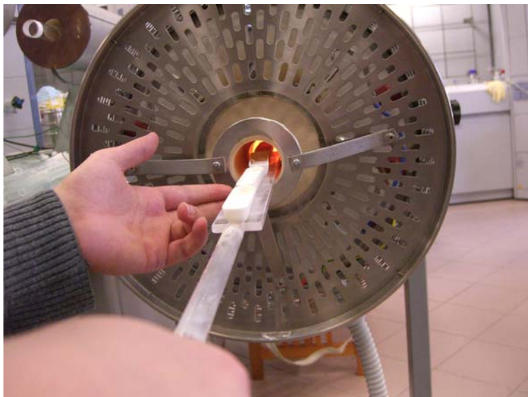
Figure 2.8 Annealing process in the tube furnace under hydrothermal conditions.
