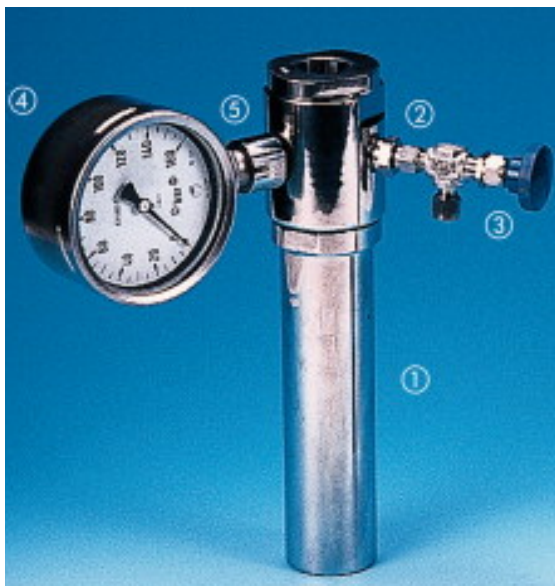
Figure 2.4: The basic equipment of Roth high pressure laboratory autoclave Model II 1) autoclave cylinder, 2) autoclave head, 3) fine control valve, 4) pressure gauge and 5) temperature sensor.
