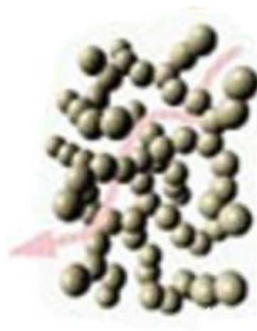
Figure 4.5 [12] Diffusion through the open pore structure of the silica aerogels
