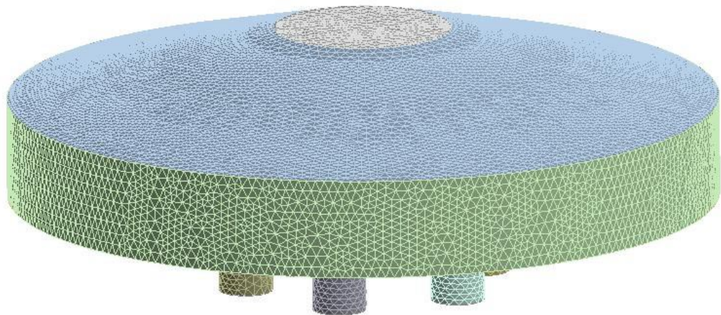
Figure 9: Surface-meshed impeller geometry in CFX-Mesh
