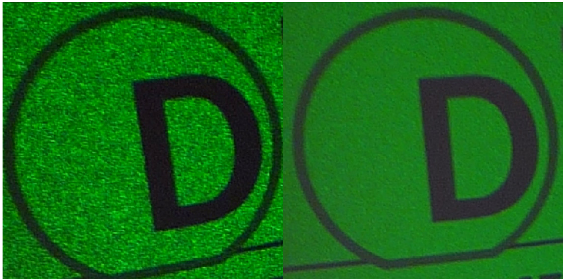
Figure A.2 Speckle on images produced by a monochrome DLP engine (left) and the effect of Dyoptyka's speckle reduction technology (Photo courtesy of Dyoptyka)
