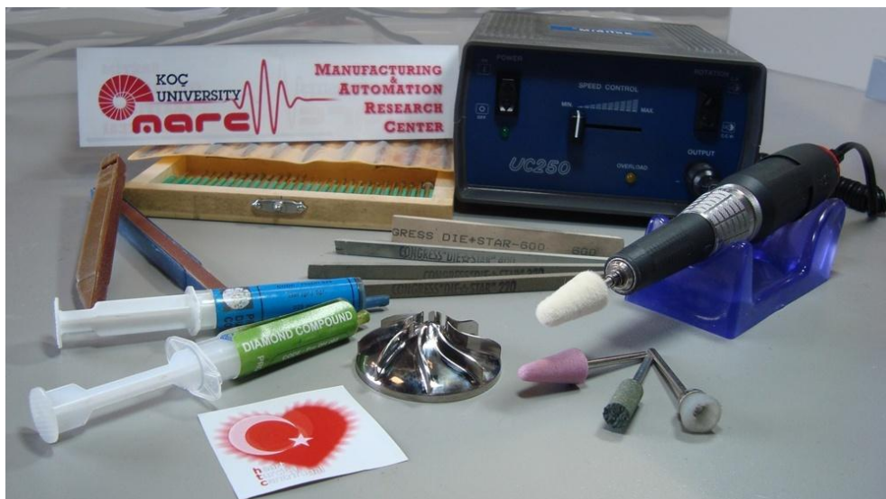
Figure 4.7 - Rotary polishing equipment with various head and polishing stones that were used
