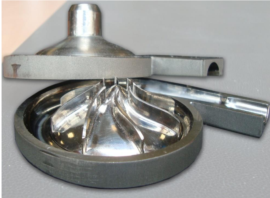
Figure 3.4 - First prototype of HTC made of Ti-6Al-4V for in vitro blood tests
