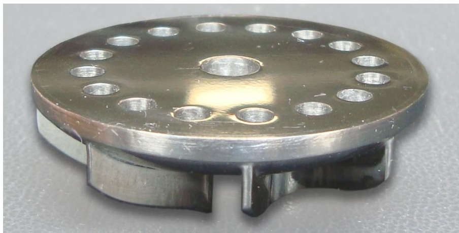
Figure 3.9 – Bottom side of the impeller where the neodymium magnets are placed
