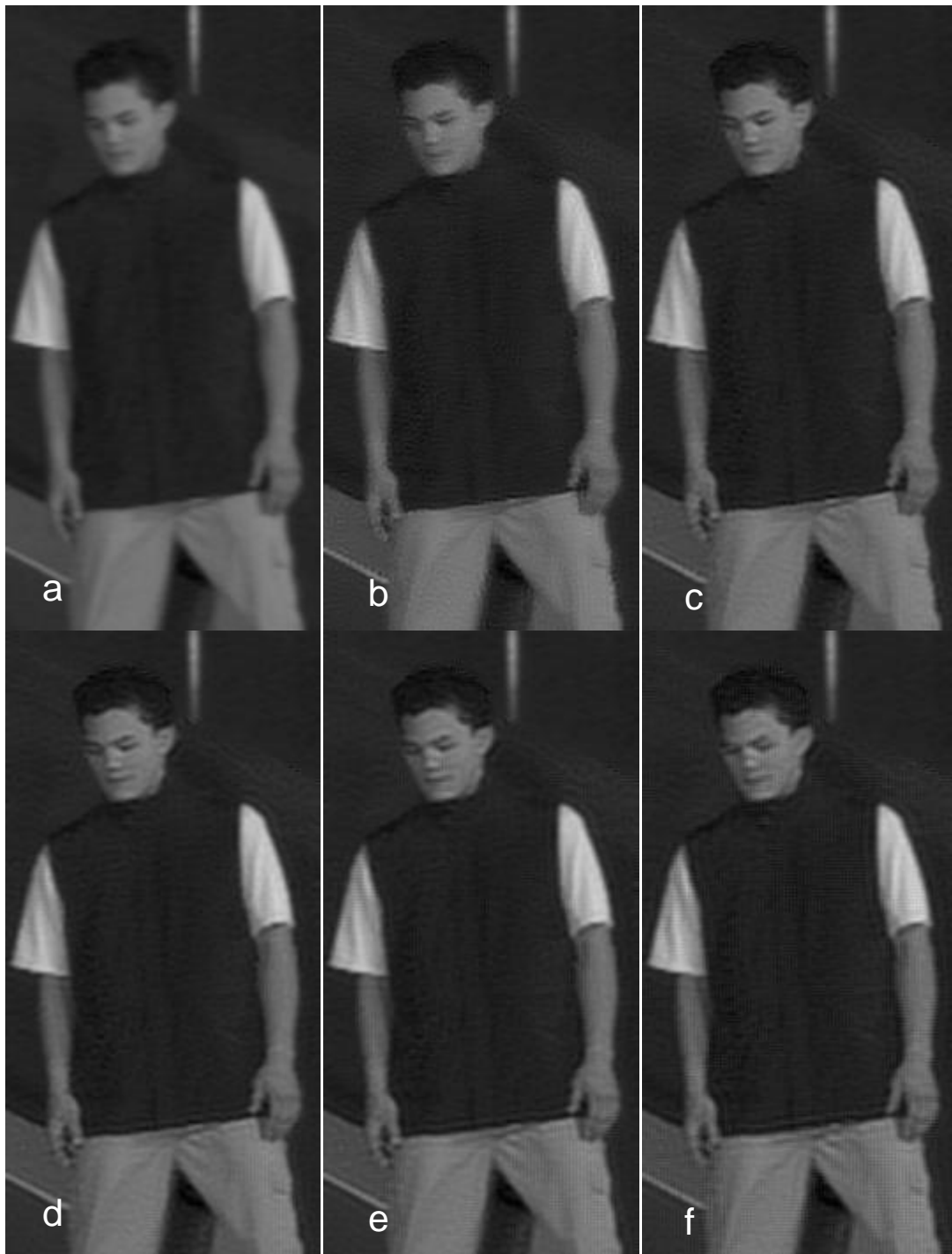
Figure 17: Effect of \sigma_{\text{psf}} parameter on SR; (a) Bi-cubic interpolation, (b) \sigma_{\text{psf}}=1.1 , (c) \sigma_{\text{psf}}=1.3 , (d) \sigma_{\text{psf}}=1.7 , (e) \sigma_{\text{psf}}=2.1 , (f) \sigma_{\text{psf}}=2.3 .
