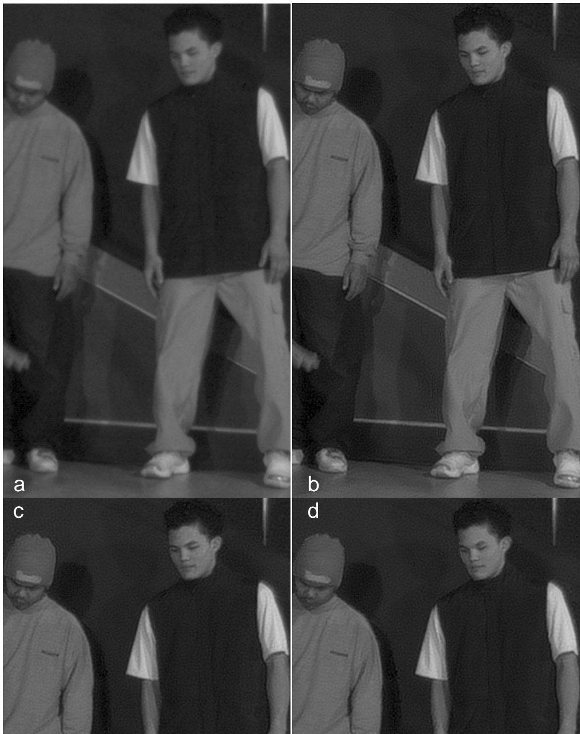
Figure 16 – Set 2 SR Results: (a) Bicubic interpolation (b) SR-proposed method without any parameter initialization, (c) SR-parameters initialized from calibration matrices (d) SR-by using motion from calibration only.
