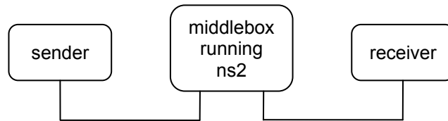
Figure 3.4 Controlled LAN test setup
