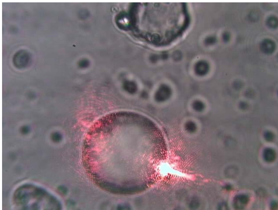
Figure 1.2. Red illuminated microdroplet under microscope. Reflection on the left is caused by the total internal reflection from the inner surface of the droplet.
