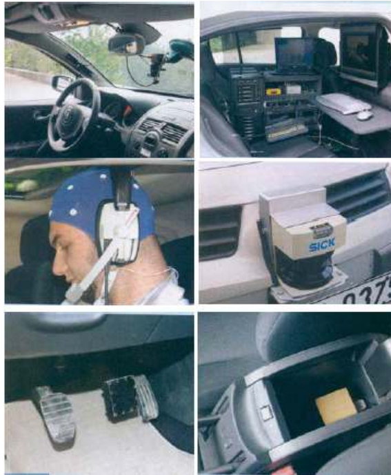
Fig. 2.1 Sensors in the data collection vehicle upperleft clockwise: cameras, navigator area and lab bench for data acquisition systems, laser scanner, IMU XYZ accelerator, break pedal pressure sensor, headset/mics, and EEG cap [13]
